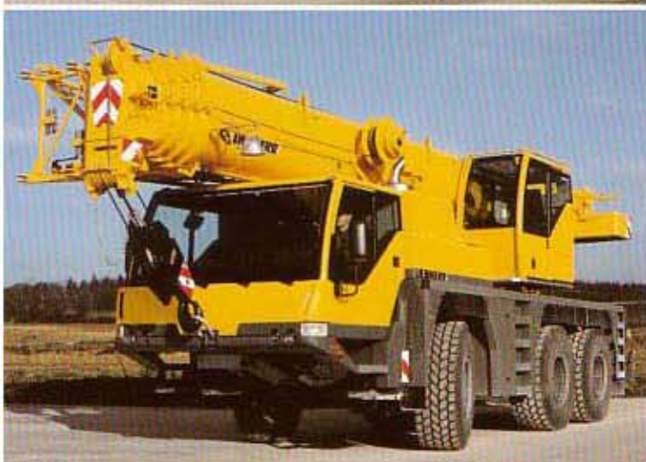
Mobile crane LTM 1055/1, max. lifting capacity 55 tons, with LI-AS-DRIVE.
