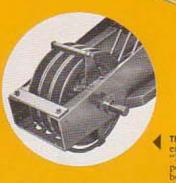
THREE SHEAVE HEAD MACHINERY for either standard angle boom or optional "HI-LITE" boom features three boompoint sheaves mounted on anti-friction point sneaves mounted on anti-friction bearings. No need to lower boom for daily greasing. Triple sheaves permit mul-tiple reeving of hoist line for extra line control in spotting loads. Jib peak sheaves also on anti-friction bearings.
