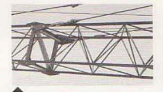
MIDPOINT SUSPENSION CABLES — This ca-ble arrangement furnished with "HI-LITE" boom gantry lends support to extra long booms at mid-point . . reduces boom de-flection when raising boom from ground. Required with all "HI-LITE" booms over 130 feet long and optional for use with
