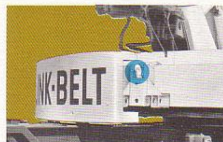
Counterweight Hydraulically Lowered/Raised
