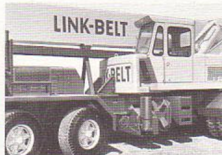
Counterweight Stored On Carrier Deck
