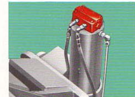
Outrigger Check Valve (Cover Removed)
