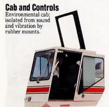
All tinted and tempered safety glass windows. Slide-by-door opens to 3'0" (0.91 m) width. Six-way adjustable operator's seat. Joy stick controllers for swing, winches and boom hoist. Foot controls for swing brake and boom telescope.
