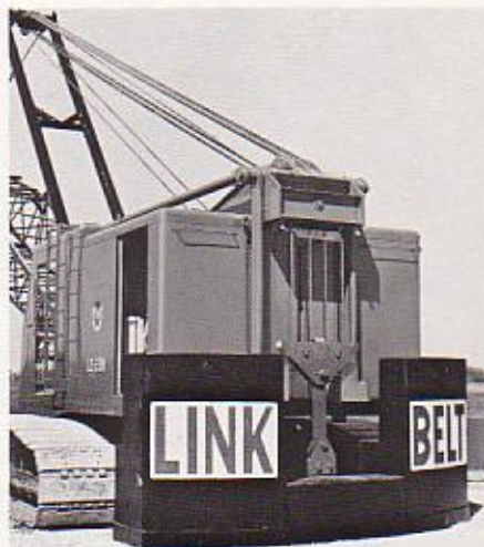
Counterweight lowering: Counterweight raising and lowering are accomplished through rope mechanism anchored to special drum on boomhoist drum shaft. Two large T-bolts hold counterweight to machine.
