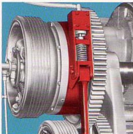
Two-speed, planetary driven hoist/lowering rope drum
