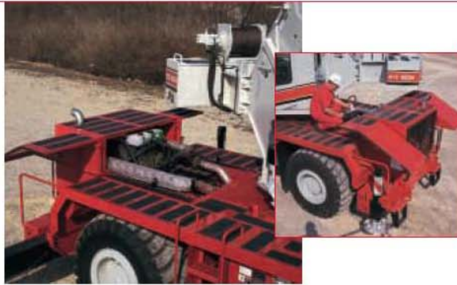
The Series II carrier is equipped with many outstanding features, making it the most "user-friendly" rough terrain crane you'll ever own. Some of the features include fold-up steps and hand rails at six points of access, non-slip surface strips on the carrier's deck and a newly designed swing-out engine hood provides quick and easy engine access for routine service.
