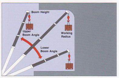
As shown in the illustration, the Automatic Moment Limiter can also be used to limit boom height, upper and lower boom angles and working radius.
