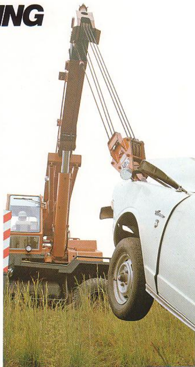
Dragging with the boom and crane winch
