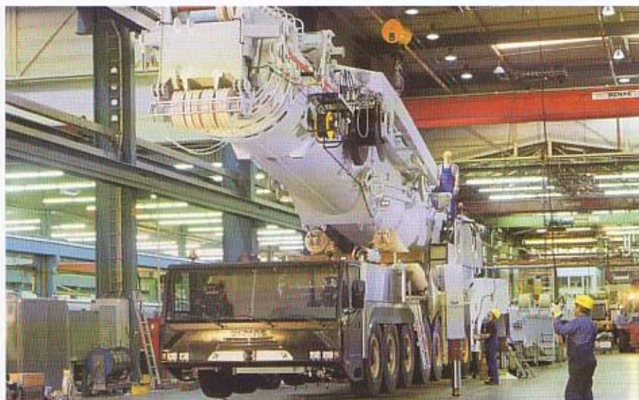
Assembly of a large telescopic crane.
